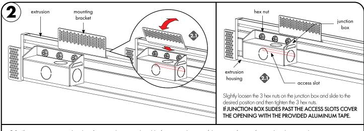
2.1 If necessary mounting brackets & junction box are adjustable if getting in the way of the support frame reference line drawings above.
