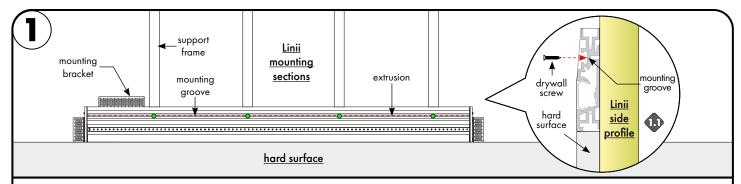
1.1 Determine the location of the installation, and then secure extrusion(s) to the support frame using drywall screws. Screws should be fastened every 16-18" depending on support frame and also at the ends of extrusion. Follow diagram above for additional information. Make sure screw is fastened through mounting grooves on the extrusion housing. Mounting brackets should be used when support frame not available. (reference step 4 for more details).
